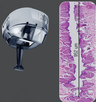
120 tip: 60mJ Depth: 952 \mu\text{m}
